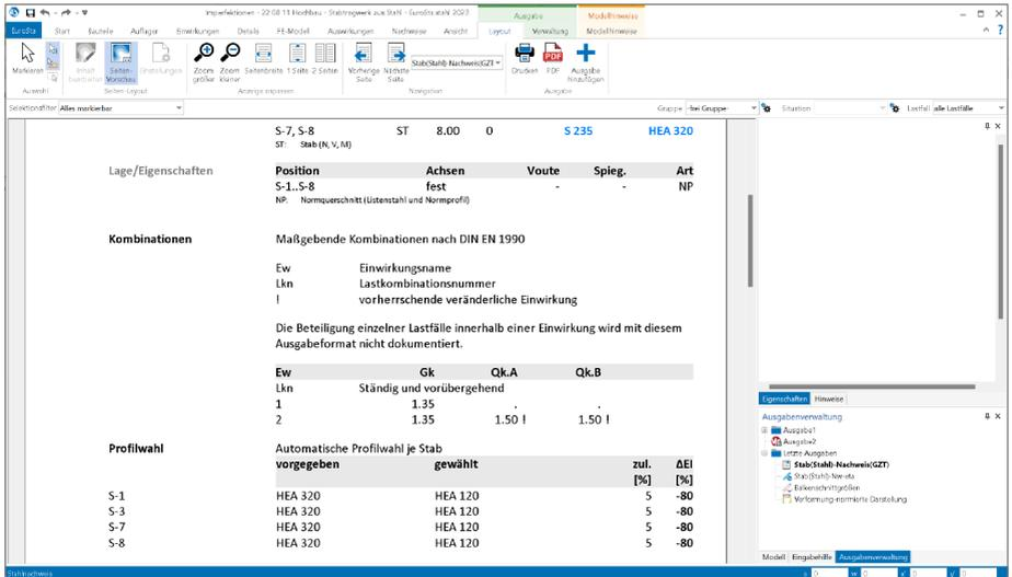
The screenshot shows the EuroSta software interface. The main window displays the configuration of a load combination. The 'Kombinationen' section shows the following table:
